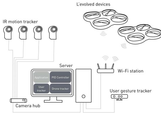
Figure 5: System configuration.
