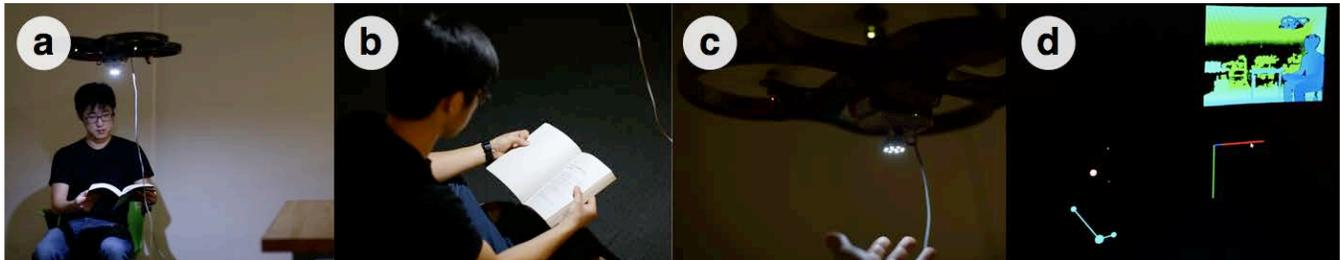
**Figure 1:** *L'evolved* lamp system. a, b) The lamp follows a user and lights up to help reading in the dark. c) Drone technology allows free 3D motion of the lamp. d) The user's activity in space is captured using a depth camera based tracking setup.
