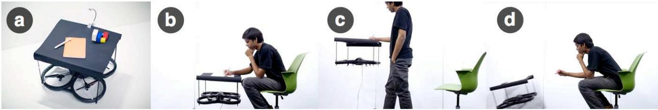
**Figure 3: L'evolved desk system. a) The desk is implemented using a drone attached to a desk surface. b, c) The desk adapts to a user's postures or walking direction. d) Auto-eject capability adds alarming or preventive function to the table.**
