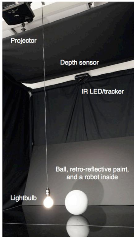
**Figure 2.** The setup of our installation
