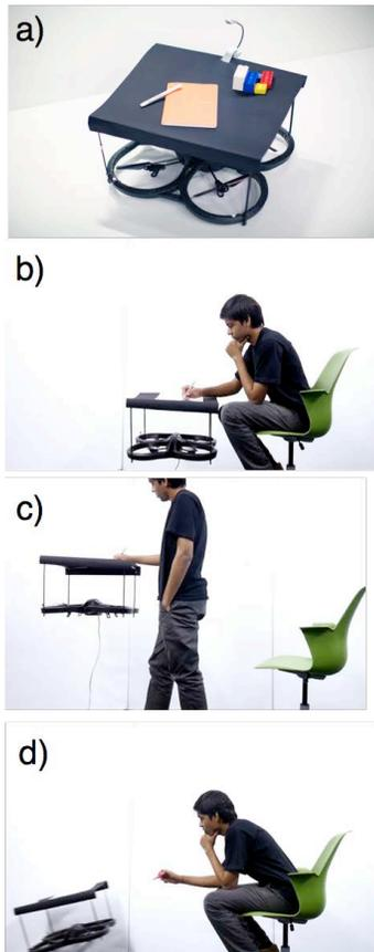
**Figure 3:** L'evolved desk system. a) Implemented using a drone attached to desk surface. b,c) The desk adapts to user's posture or walking position. d) Auto-eject capability adds preventing or alarming functionality to table
