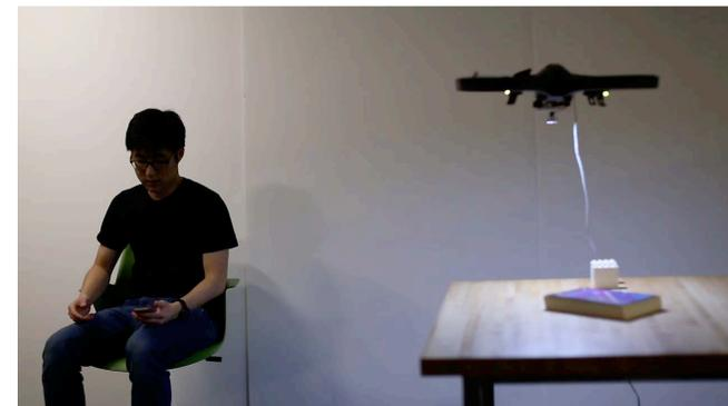
**Figure 1:** A lamp can direct a user's attention to a location or an object of interest. It can memorize the last location of a book the user was reading, and shed light on it upon the user's request
