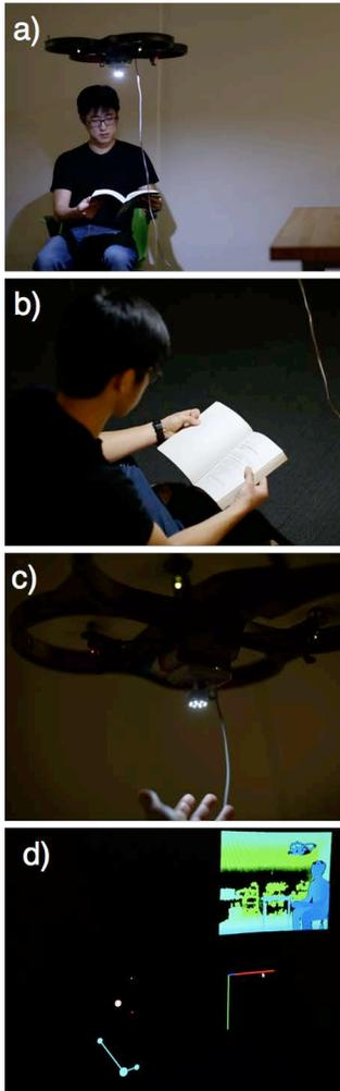
**Figure 2:** L'evolved lamp system. a,b) The lamp follows a user. c) Drone technology allows free 3D motion. d) User's activity is tracked using a depth camera
