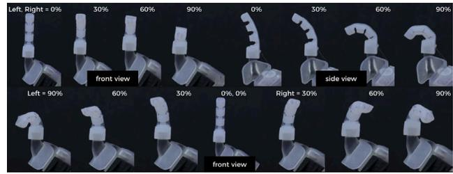
**Figure 4: Front and side view of the tendon driven control. The use of two tendon wires allows for expressive control of the robot in 2D control space.**
