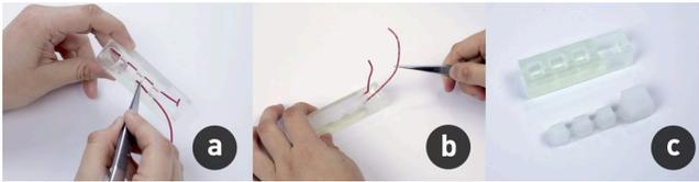
**Figure 3: Fabrication process of the robotic fingers. a) channels are created by threading wires into the mold. b) after curing, the wires are pulled out to leave the channel open. c) final casted finger piece.**
