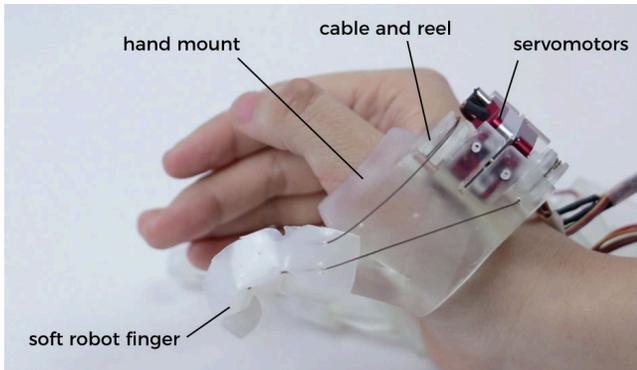
**Figure 2: Configuration of our system. The servomotors are mounted on the back of the hand attachment module, pulling the strings for robotic control.**
