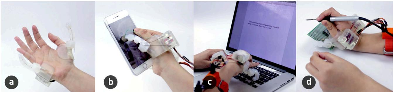
**Figure 1:** a) The configuration of our system. b) performing multi-touch gesture with the soft robotic finger. c) the soft robotic finger supports keyboard typing. d) the fingers can hold and adjust the position of an object in tri-manual tasks.
