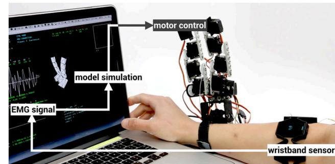
**Figure 1:** Sensor, control software, and the joints interface.
