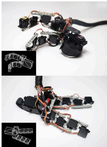
**Figure 2:** Our hardware. 11 motors are linked using LEGO parts, each of them with 180 degrees motion range. The wireframe diagrams illustrate the overall structure. Cables from each motor are connected to an Arduino controller.
