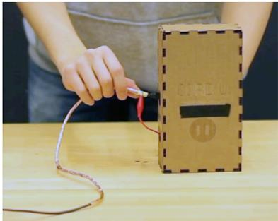
Figure 1: Sliding one's fingers along the cable or applying pressure can be used to control *data flow*
