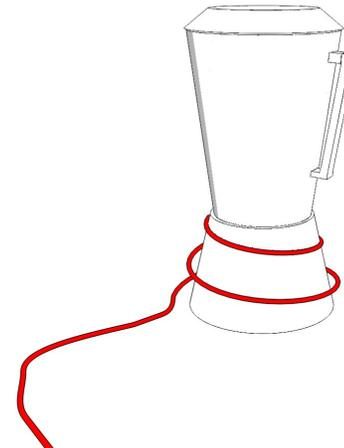
Figure 5: Cable wrapped around blender as speed control
